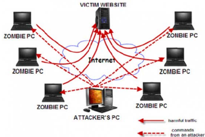
Figure 4: Sample Configuration of a DDoS Attack 21
